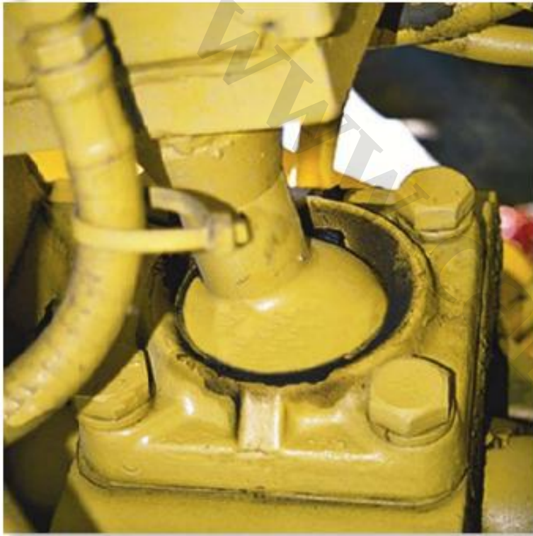
This ball-and-socket joint provides a connection for the housing of an earth grader to its frame
